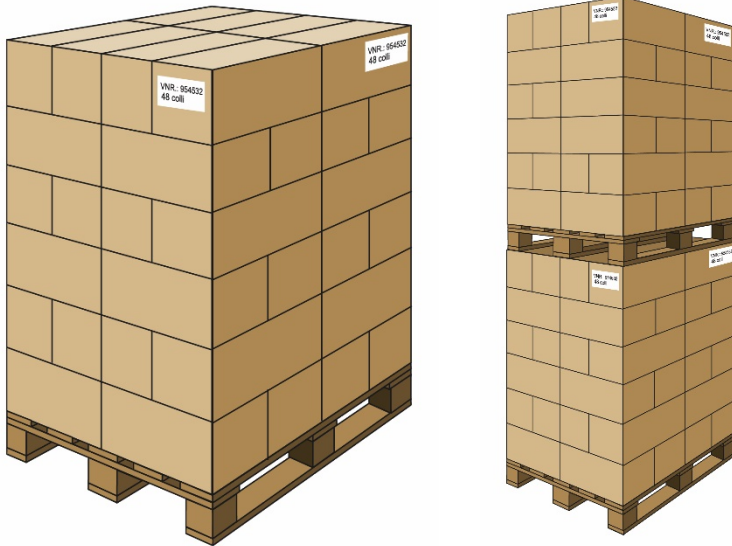
Figure 11: - Examples of a perfect way to pack a pallet, with the boxes in joint-break arrangement, for stability when foil is removed
